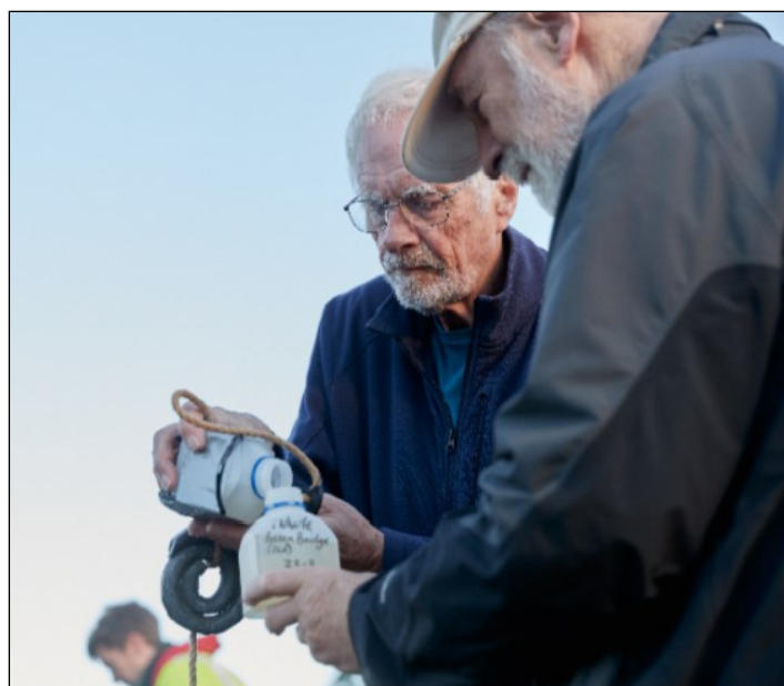
Sampling for faecal bacteria using sterilised containers
